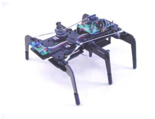
Figure 4. The Lynxmotion Hexapod 1 (OOPic-R) Kit [26].
