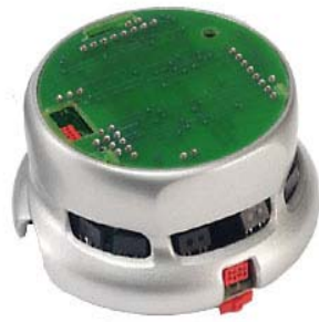
Figure 6. The K-Team Khepera II minirobot kit [21].
